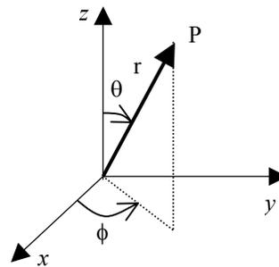
Fig. 2 Spherical coordinate system
